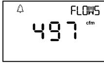
The Flow parameter appears. This parameter represents the airflow as measured by the controller.
