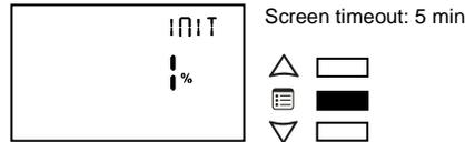
The damper begins the initialization process. During this process, the screen displays -1.
