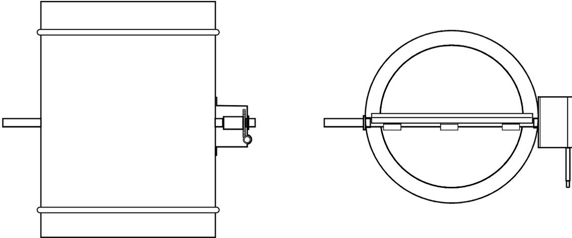
The SC-FS-CBD-XX is designed to provide efficient airflow control in conventional air handling systems. It consists of a round damper with a locking worm gear regulator.
