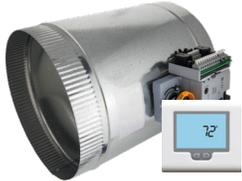
The Zone One is an SC-ZD stand-alone control damper assembly designed to solve over-heating and over-cooling problems. It can be used to control a single room, or parallel multiple dampers to modulate air flow in multiple rooms. Each zone requires an SC-Z20-T and can be paralleled to SD Series dampers if needed. The SC-ZD features a 24VAC, 2VA floating-point actuator (45 lb-in).
