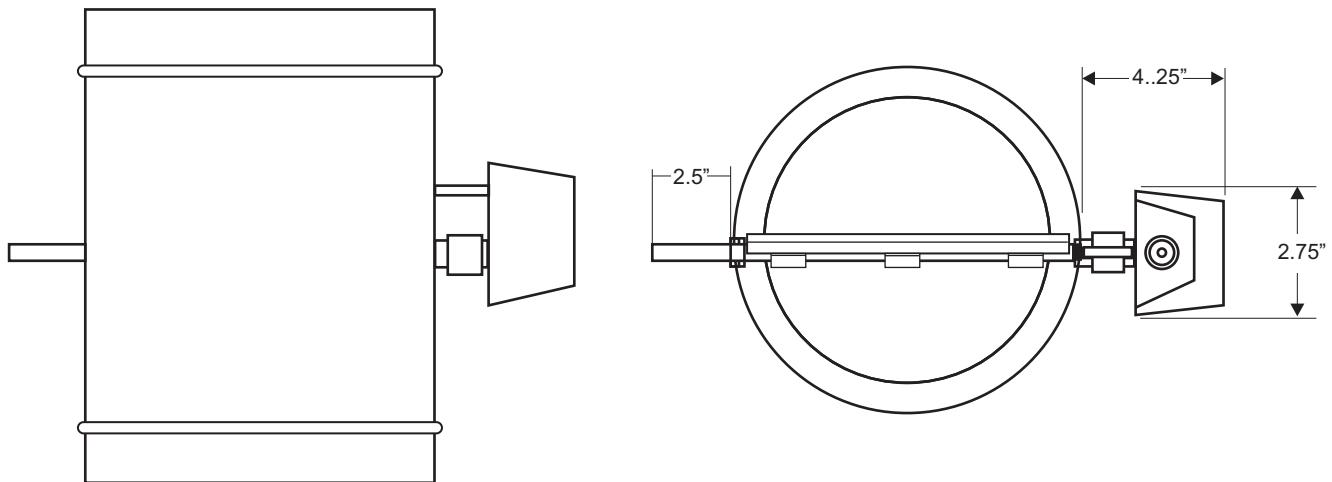
The SC-OAD-XX is designed for retrofit or new construction applications requiring exhaust, fresh air intake and on-off zone control. Typical application use includes bathrooms or restrooms in high rise hotels, office buildings and apartment buildings. The damper includes a direct coupled, spring return actuator available in 24 VAC or 110 VAC . Made in the U.S.A.
